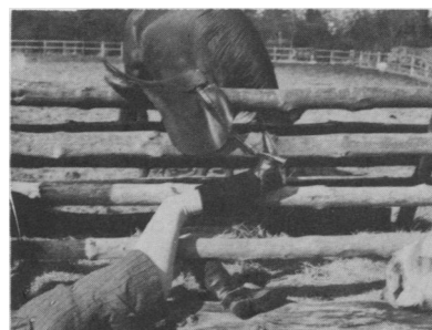
This mock fall shows how this riding boot cannot go through the stirrup. The foot tends to fall from the stirrup as soon as the rider hits the ground.
