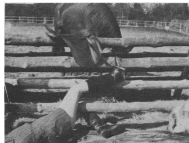
This mock fall shows how this riding boot cannot go through the stirrup. The foot tends to fall from the stirrup as soon as the rider hits the ground.
