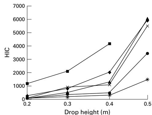
Figure 2 Head injury criterion (HIC) *v* drop height for six models of rigid headform. The results for two models were omitted to keep the scale in proportion with an HIC of 1000 as the standard pass/fail criterion.
