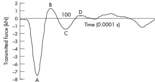
**Figure 3** Forces within impacts on standard EVA mouthguard material without air inclusions.
