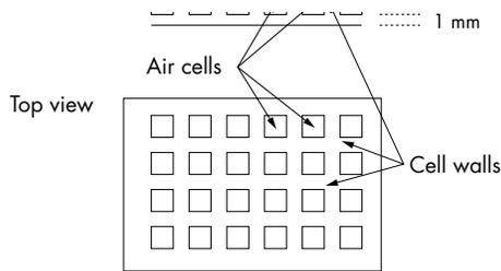
**Figure 2** Construction of air inclusion materials.
