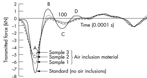
**Figure 4** Forces within impacts on EVA mouthguard materials with and without air inclusions.
