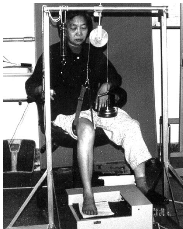
Figure 1 Testing apparatus and a subject positioned for evaluation of passive movement sense of ankle.
