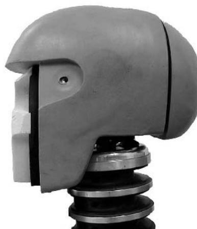
Olympic headgear was placed on the dummy, but the blows were straight to the face and did not engage the headgear. For positioning, the upper torso was attached to a rigid table with a foam pad placed below the Hybrid III abdomen insert so that the dummy remained in an upright position during the impact.
