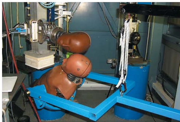
Figure 6 Head to head impact test set-up (front boss to side). Note that the falling head (upper) gets fitted with the headgear, and the lower head/torso may rebound naturally on impact.
