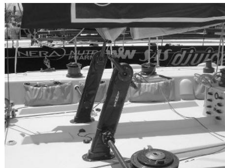
**Figure 2** Pedestal winches for grinding.
