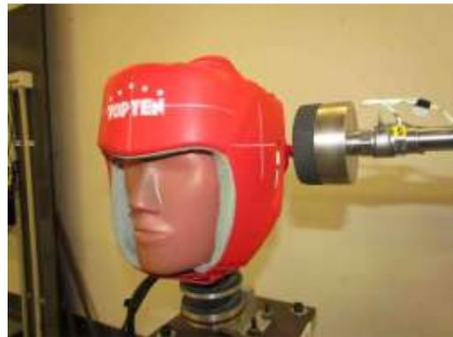
**Figure C2: Left lateral impacts with disc-pad interface.**
