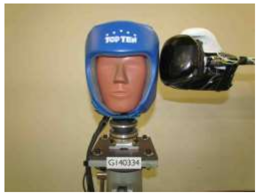
Figure C3: Centre-front forehead and lateral impacts with glove-fist interface.
