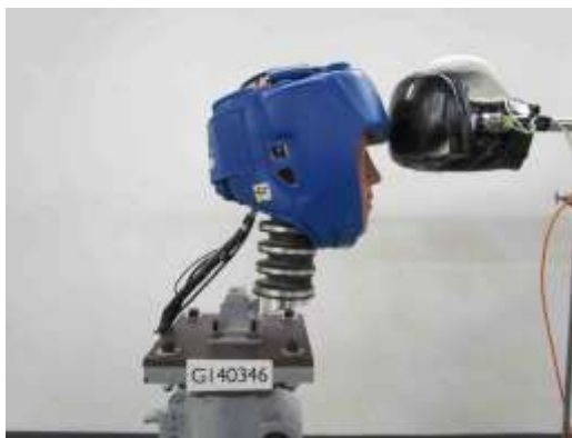
Figure C3: Centre-front forehead and lateral impacts with glove-fist interface.
