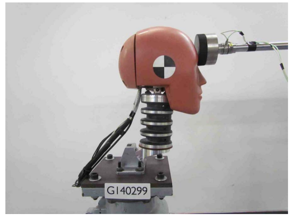
Figure 2 Hybrid III head and neck configuration. Frontal impact condition shown. The head orientation was checked before each test. The SAE J211 sign convention was applied: +x=anterior; positive rotation around x is right lateral flexion (also referred to as roll); +y=lateral right; positive rotation around y is extension (referred to as pitch); and, +z=inferior; positive rotation around z is right rotation (also referred to as yaw).
