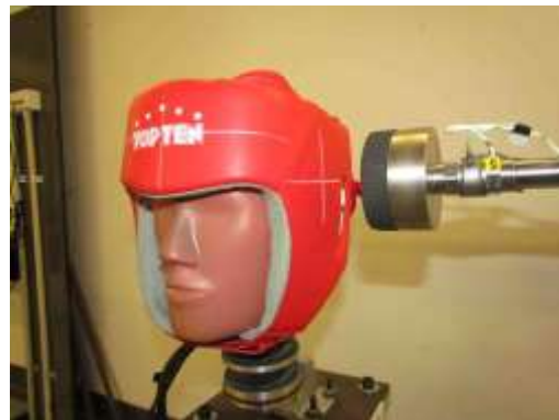
Figure C2: Left lateral impacts with disc-pad interface.
