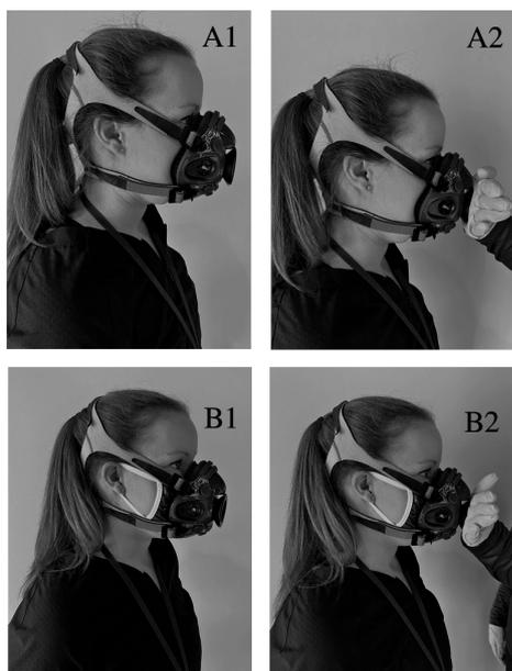
**Figure 2** Fit comparison of K5 COSMED masks with and without cloth face masks. (A1) K5 COSMED mask with no cloth face mask; (A2) K5 COSMED mask with no cloth face mask during fit test; (B1) K5 COSMED mask with cloth face mask and (B2) K5 COSMED mask with cloth face mask during fit test.
