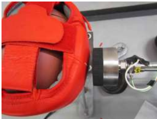
Figure C2: Left lateral impacts with disc-pad interface.
