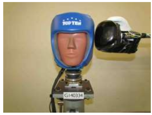
Figure C3: Centre-front forehead and lateral impacts with glove-fist interface.
