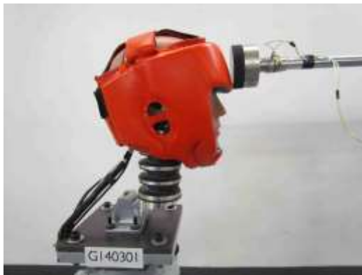
Figure C1: Centre-front forehead impacts with disc-pad interface. There is some parallax error in the photographs that suggests that the impactor was not aligned horizontally. The impactor was aligned horizontally in all tests.
