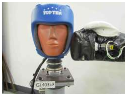
Figure C5: 60° jaw impacts. The impact axis was aligned to be 60° from the mid-sagittal plane measured in the horizontal plane.
